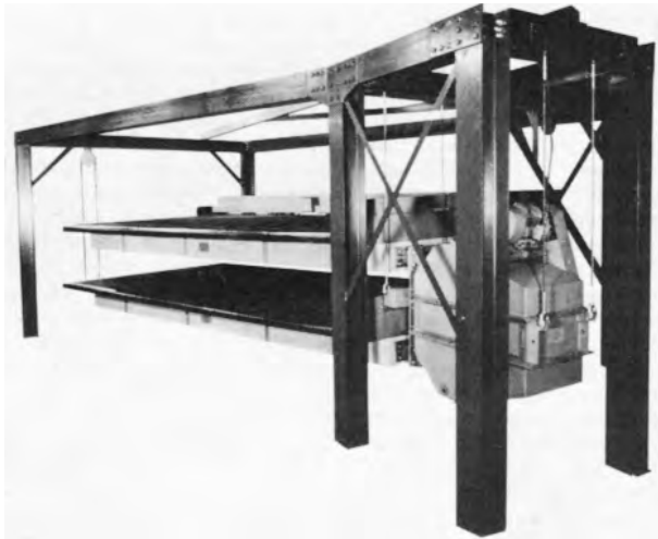
FIG. 19-29 Two-deck concentrating table. (Courtesy Deister Concentrator Company, Inc.)
