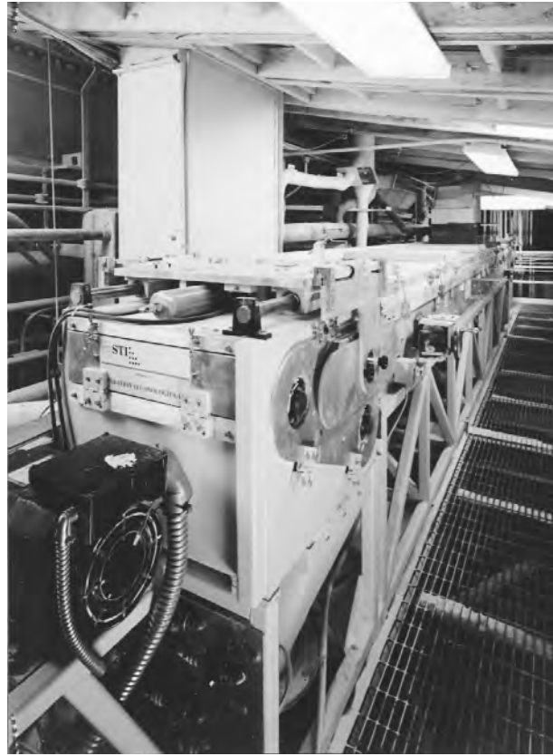
FIG. 19-58 Triboelectric separators. Belt-type electrostatic separator for separation of carbon from fly ash. (Courtesy of Separation Technologies, Inc.)
